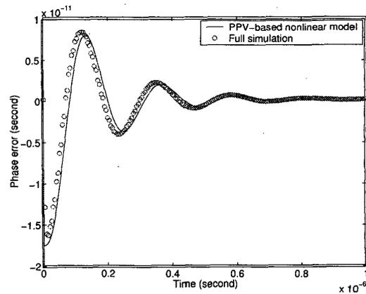
Fig. 5. The impulse response of the PLL
