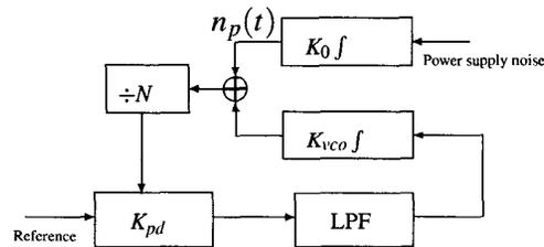
Fig. 1. Functional block diagram of a PLL.
