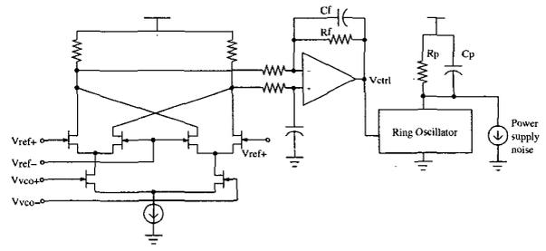
Fig. 3. Diagram of ring-oscillator based PLL.
