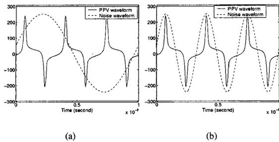
Fig. 7. (a) The PPV and the power noise with the frequency  $f = 1.01f_0$ . (b) The PPV and the power noise with the frequency  $f = 3.03f_0$ .
