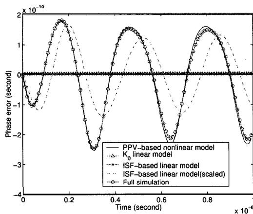
Fig. 8. The phase error due to supply noise with the frequency  $f = 3.03f_0$
