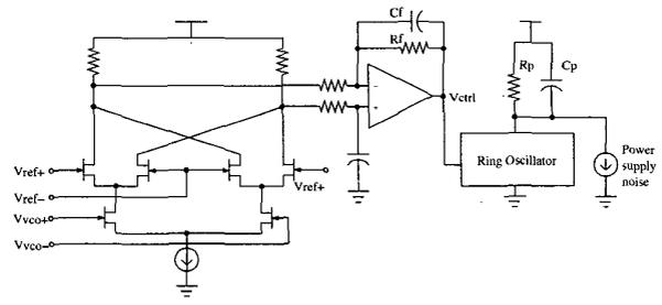
Fig. 3. Diagram of ring-oscillator based PLL.
