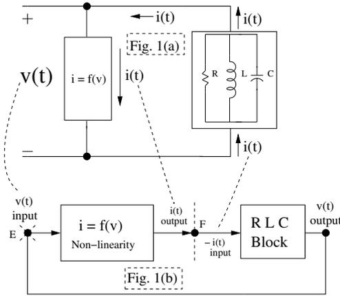
Figure 1: Generic LC oscillator circuit
