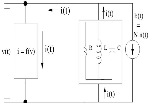
Figure 3: Generic Oscillator with noise
