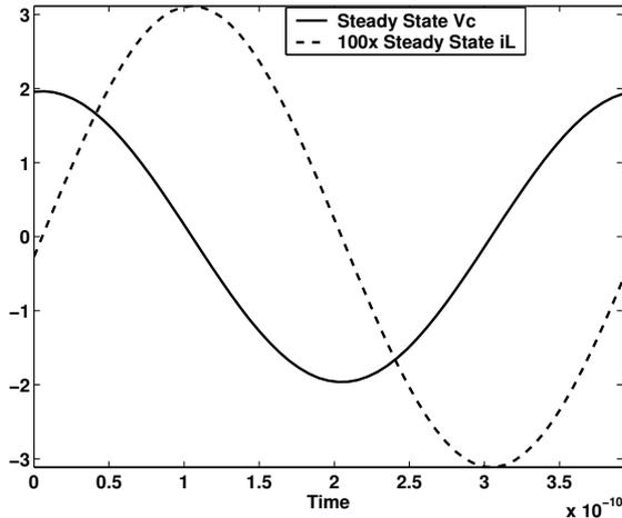
Figure 4: SS voltage  $v(t)$ , current  $i_L(t)$  - CMOS oscillator
