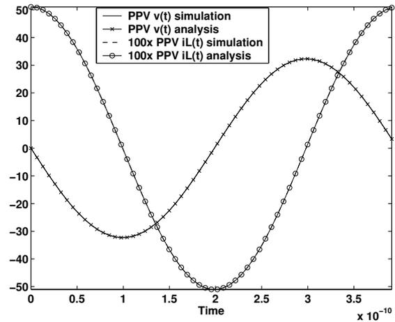
Figure 6: Simulation for PPV - 3 Components - CMOS oscillator
