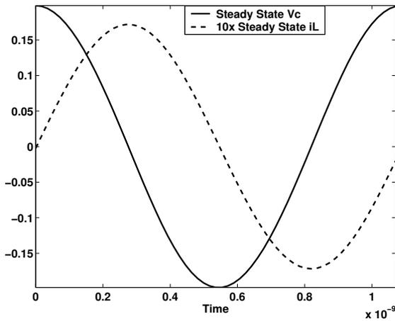
Figure 7: SS voltage  $v(t)$ , current  $i_L(t)$  - tanh oscillator
