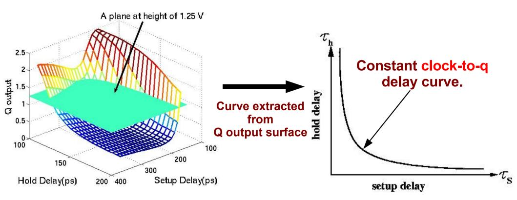
Q value vs setup and hold delays
