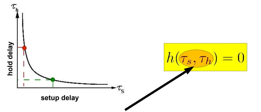
A scalar equation with two unknowns (setup & hold time)
