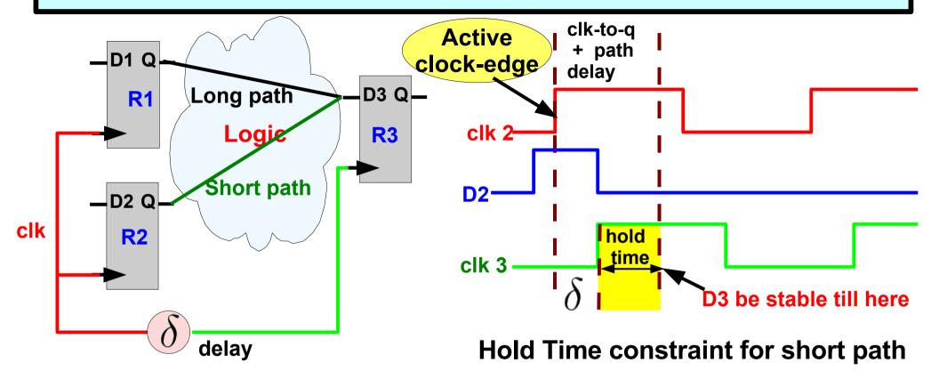
hold-time<sub>R3</sub> +  $\delta$  < clk-to-Q-delay<sub>R2</sub> + short-path-delay
