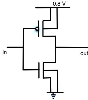
Fig. 5. Inverter circuit.
