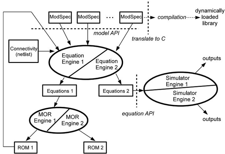
Fig. 4. Schematic description of the model compilation procedure.
