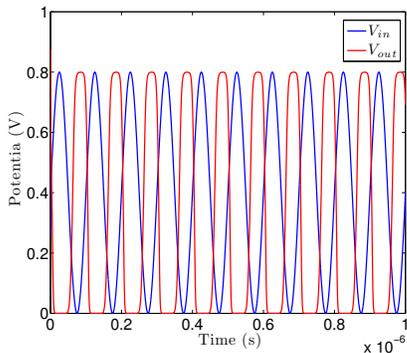
Fig. 6. Inverter circuit output under a sinusoidal input.
