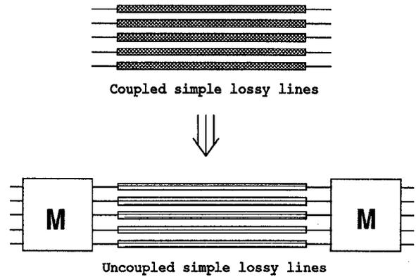
Figure 4: Multiconductor Decomposition
