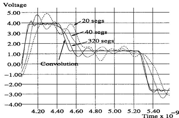
Figure 3: Lumped-RLC method, varying no. of segments
