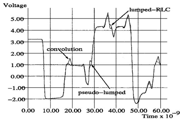
Figure 5: raytheon1 receiver-end voltage
