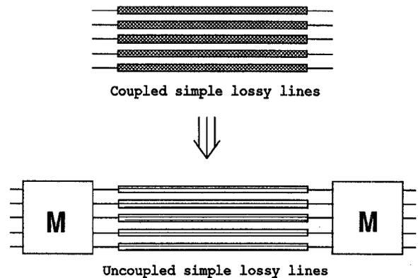
Figure 4: Multiconductor Decomposition
