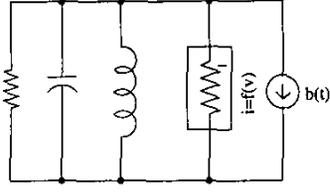
Fig. 1. A simple LC oscillator.
