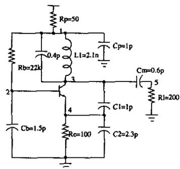
Fig. 11. A 4GHz LC oscillator.
