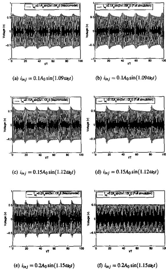
Fig. 9. Outputs of the simple ring oscillator under various perturbations.
