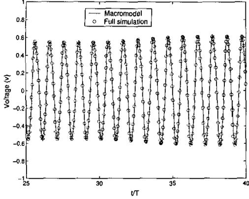
Fig. 4. Output of the simple LC oscillator under the perturbation  $i_{inj} = 0.05A_0 \sin(1.03\omega_0 t)$ .
